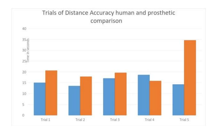
This chart shows the comparison of human times to the prosthetic in distance accuracy. This task is how fast you can throw three different ball types into a bucket at different ranges. The ball types consist of tennis balls, ping pong balls, and hacky sacks. The objective of this is to make at least one of each ball type in the shortest time possible.
